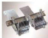
钢丝绳断裂保护装置 在钢丝绳断裂时,卡阻轨道,门体不 下垂 Cable break device The rail is jammed and the door body does not fall in the event of broken wire rope
